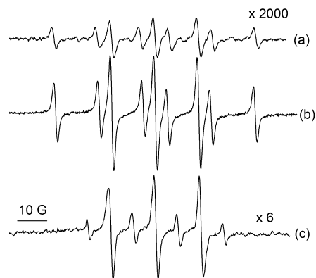
Figure 1. EPR spectra of H spin adducts formed during aerobic oxidation of secondary alcohols over supported and unsupported gold catalysts: (a) DMPO-H adduct for AuPPh 3 nanoparticles and 2-pentanol, (b) DMPO-H adduct for Au/CeO 2 and 3-octanol and (c) PBN-H adduct for Au-PI and 1-phenylethanol.
